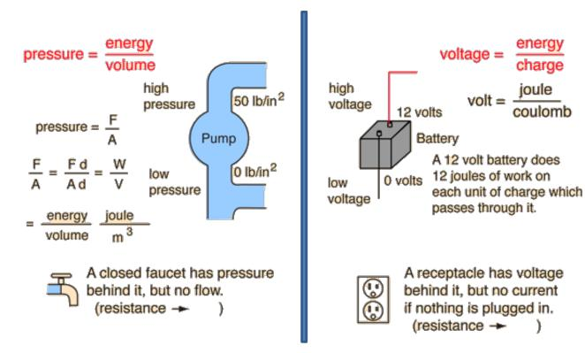
A battery takes charge, does work on it, then releases it at high potential energy. **It does not create or provide charge, it merely pumps the charge already in the wires.**
